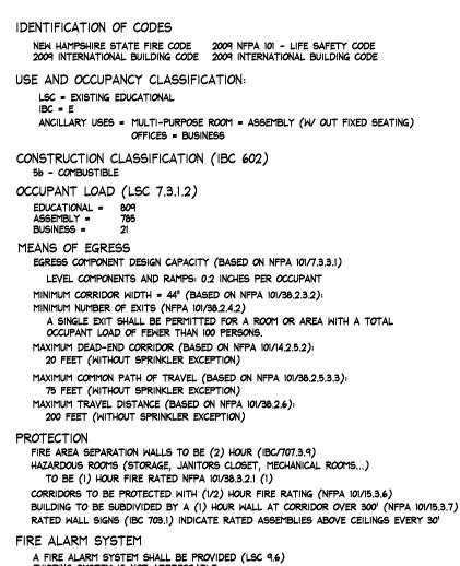
A FIRE ALARM SYSTEM SHALL BE PROVIDED (LSC 9.6) EXISTING SYSTEM IS NOT ADDRESSABLE EXISTING SYSTEM DOES NOT HAVE VOICE EVACUATION IN ASSEMBLY AREAS
