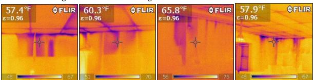
Image 13: Outside air leaking into interior walls from the attic
