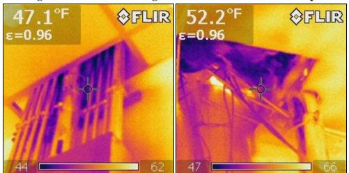
**Image 7: Penetrations through the attic into the conditioned space**
