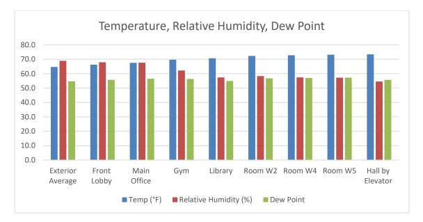
Temperature will affect the occupant's perception of IAQ based on employee comfort levels, effect of drafts or airflow, and humidity levels in a building. In most cases, simple adjustments to thermostats and direction of airflow from registers can improve perceived
