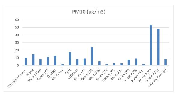
These results indicate that the HVAC filters are not reducing the overall particle loading inside the building when compared to the outside air. The US EPA does have a National Ambient Air Quality Standard at 150  $\mu$ g/m<sup>3</sup> which was not exceeded during the testing. The World Health Organization (WHO) also has set a standard of 50  $\mu$ g/m<sup>3</sup> as a 24-hour average and 25  $\mu$ g/m<sup>3</sup> as an annual average exposure.
