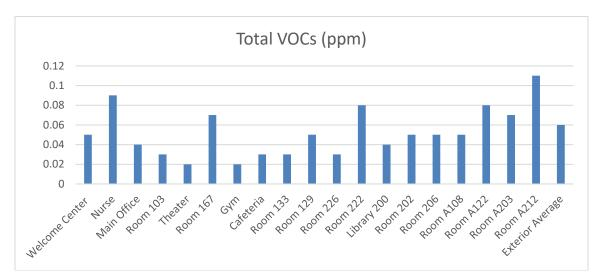
The U.S. Environmental Protection Agency (EPA) reports that levels of volatile organic compounds (VOC) are almost always higher indoors compared to outdoors. Based on past testing, total VOC readings of up to 1 ppm are not atypical in general IAQ settings. In addition, the American Industrial Hygiene Association (AIHA) Technical Committee on Indoor Environmental Quality 1993 publication indicates that a general acceptable range for indoor air total VOC screening is less than 1.0 ppm.
