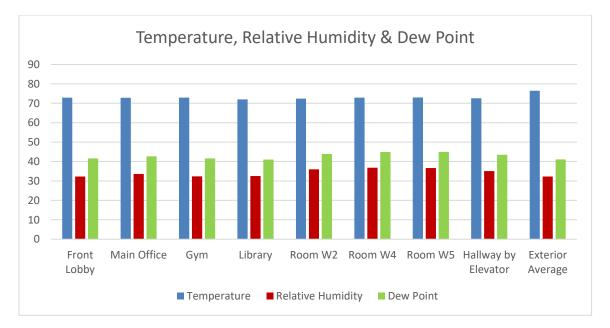
Temperature will affect the occupant's perception of IAQ based on employee comfort levels, effect of drafts or airflow, and humidity levels in a building. In most cases, simple adjustments to thermostats and direction of airflow from registers can improve perceived
